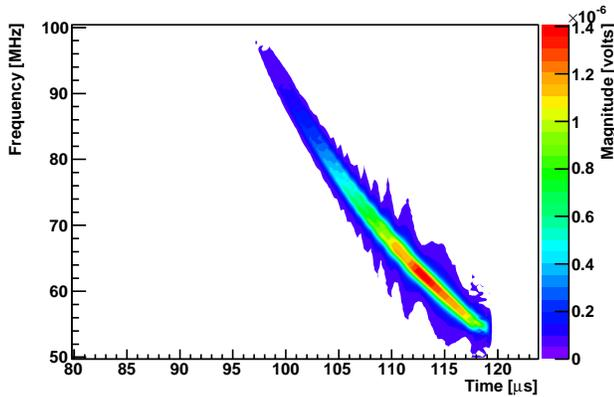
**Fig. 2:** Spectrogram of “chirp” for simulated air shower, initiated by  $10^{19}$  eV cosmic ray midway between 54.1 MHz transmitter (TX) and receiver (RX), located 50 km apart. The shower is inclined at a zenith angle of  $30^\circ$  in a plane perpendicular to a line connecting transmitter and receiver.
