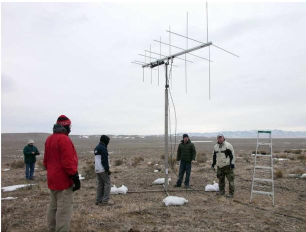
**Fig. 3:** Radar receiver antenna at Long Ridge fluorescence detector site.
