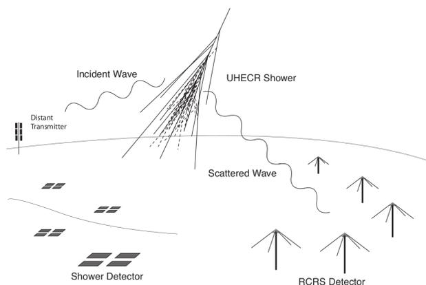
**Fig. 1: The bistatic radar technique, as pioneered by the MARIACHI experiment. Conventional surface detectors are used to tag the presence of air showers while radar receiver stations detect the forward scattered echo.**
