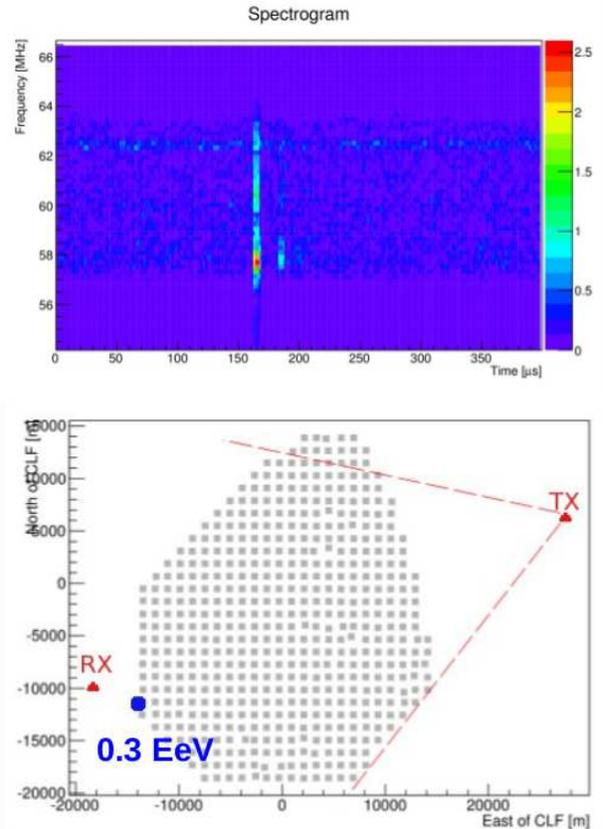
**Fig. 4:** Interesting waveform obtained in TARA1.5 FD-trigger stream. *Top:* Spectrogram. The sampling rate of the TARA1.5 receiver, 12.5 MS/s, was too slow to allow resolution of frequency changing with time. *Bottom:* Core location and energy of cosmic ray air shower which triggered the fluorescence detector.
