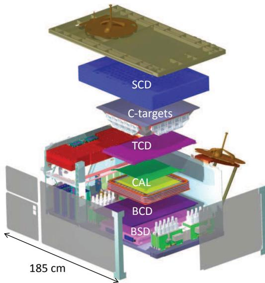
**Fig. 1:** Exploded view of the ISS-CREAM Instrument.
