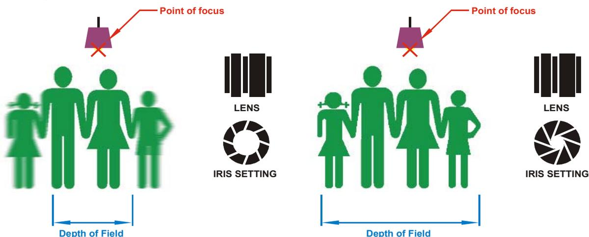
One disadvantage of increasing the depth of field by closing the iris, is the amount of light admitted to the camera will be reduced and the image will become darker. Depth of field is also dependent upon the focal length of the lens. Wide angle lenses (i.e. those with a small focal length) will have a greater depth of field than telephoto types. The depth of field is inversely proportional to the focal length of the lens so as focal length increases, the depth of field will decrease.
