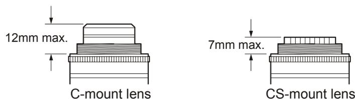
NOTE: A CS-mount lens will not work on a camera designed to be used only with C-mount lenses
