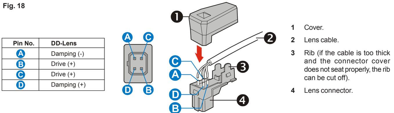
**DD Lens Level Adjustment for Fixed and Zoom Lenses**
