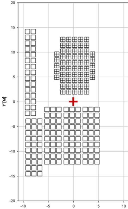
**Fig. 2:** Diagrammatical view of the underground muon carpet. Open squares – arrangement of 150 muon detectors before modernization. Crossed squares – 60 additional detectors. Central cross is the geometrical center of the GAMMA installation.
