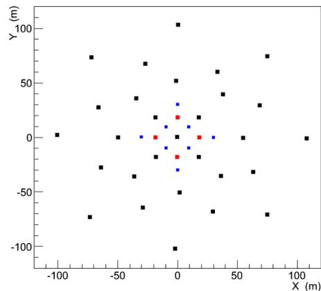
**Fig. 1:** Arrangement of the surface detector stations. Black and red squares 33 stations with 3 (or 4) of  $1\text{m}^2$  scintillation detectors in each. Blue squares, 8 stations with 1 detector in each.
