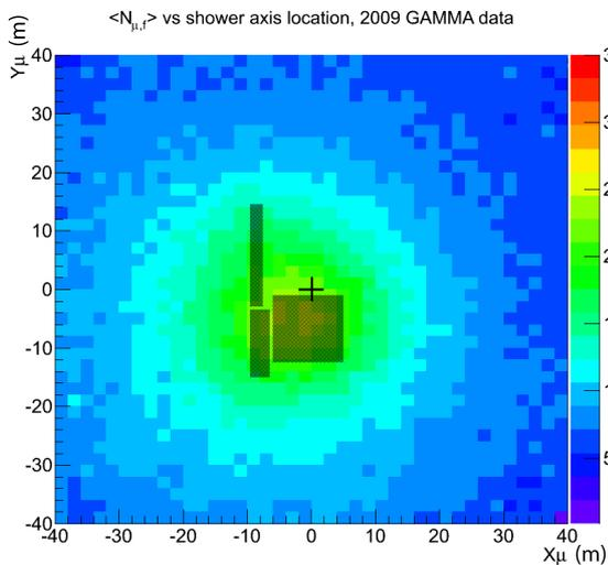
**Fig. 3:** Distribution of the average number of fired muon detectors  $N_{\mu,f}$  as a function of the shower axis position  $(X_{\mu}, Y_{\mu})$  in the muon detector plane (2009 GAMMA data).
