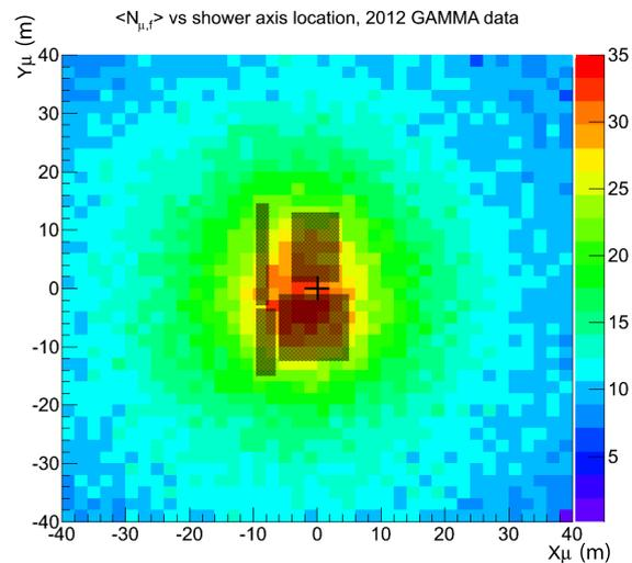
**Fig. 4:** Distribution of the average number of fired muon detectors  $N_{\mu,f}$  as a function of the shower axis position  $(X_{\mu}, Y_{\mu})$  in the muon detector plane (2012 GAMMA data).
