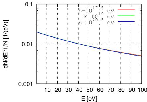
**Figure 1:** Graphical representation of the electron energy distributions as expected for electrons ionized by an incident distribution as described by Eq. (4) and Eq. (2). The plot shows the expected distribution expected at shower age  $s = 1$  for vertical showers of different energies. The differences between the curves is very small and almost impossible to see in this presentation.
