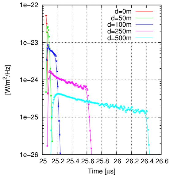
**Figure 4:** Expected signal traces given in units of spectral energy flux density at most likely distances for CROME-like events. The time coordinate is chosen such that  $t = 0$  at the point where the shower crosses  $s = 0.7$ .
