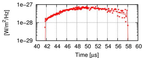
**Figure 5:** Expected signal trace given in units of spectral energy flux density at most likely distances for a MIDAS-like event. The distance from shower impact is  $d = 10$  km. The time coordinate is chosen such that  $t = 0$  at the point where the shower crosses  $s = 0.7$ . The divergence at later times is due to slight geometric instabilities caused by large cell sizes.
