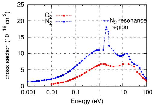
**Figure 3:** Momentum cross sections of molecular oxygen and nitrogen at low incident electron energies. The cross section of molecular nitrogen in the resonance region, as indicated, is plotted at its best estimate.
