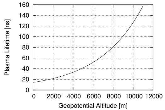
**Figure 2:** Expected lifetime of plasma with respect to altitude.
