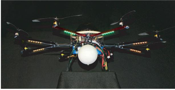
**Figure 1:** The Octocopter with the light source suspended below it. Green LEDs indicate the forward direction.
