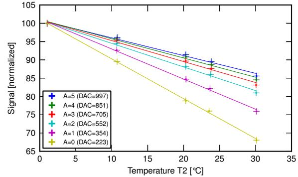
**Figure 2:** Relative signal strength from the Octocopter light source as a function of the temperature. Measurements were made at the DAC settings of the six standard amplitudes, A0 being the lowest and A5 the greatest. The amplitudes at each DAC setting are normalized to 100% at 0°C.
