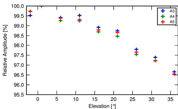
**Figure 5:** Relative signal strength from the Octocopter light source as a function of the elevation rotation angle from the forward direction. (Source amplitude settings A3(blue), A4(green), and A5(red))
