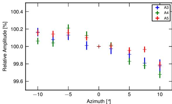
**Figure 4:** Relative signal strength from the Octocopter light source as a function of the azimuthal rotation angle from the forward direction. (Source amplitude settings A3(blue), A4(green), and A5(red))
