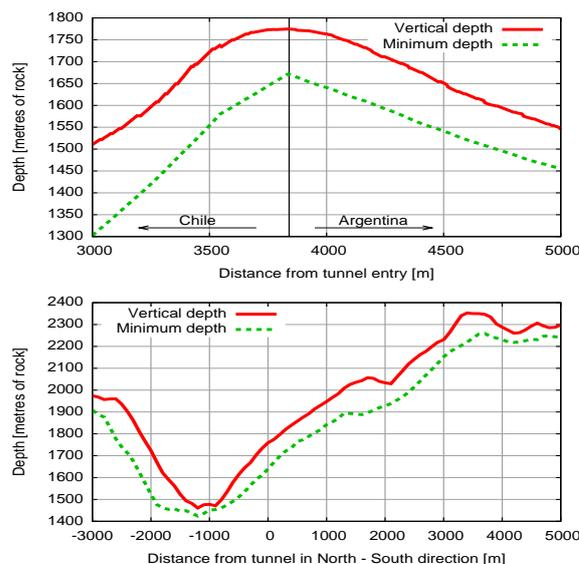
**Figure 4:** Vertical and omnidirectional minimum depth obtained depending on the location of the laboratory with respect of the tunnel. See text for details.
