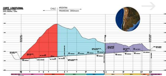
**Figure 1:** Longitudinal cut of the Agua Negra tunnel and its location.
