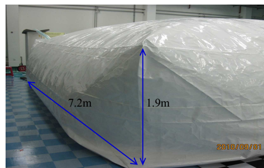
Fig. 2: One of the Tyvek bags (7.2 m in side length and 1.9 m in height) filled with air in clean hall.
