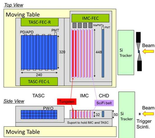
Figure 3: Configuration of the CALET prototype II for the beam test at CERN-SPS in 2011.
