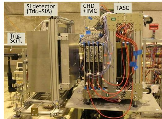
**Figure 5:** The CALET BTM was rotated by 90 degrees and set up on a moving table at H8 beam line of CERN-SPS.
