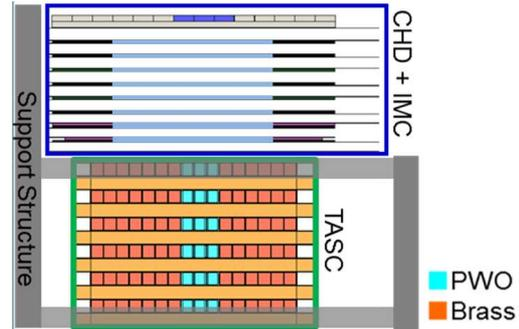
**Figure 4:** Configuration of the CALET BTM for the beam test at CERN-SPS in 2012.
