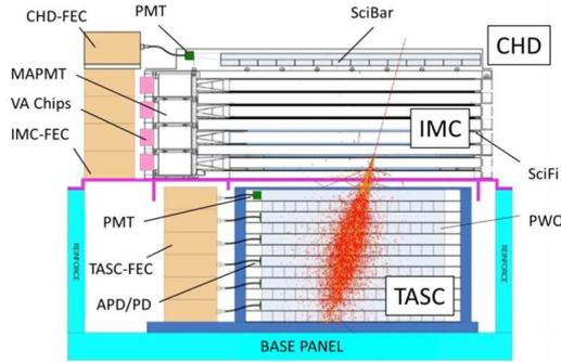
Figure 1: CALET main telescope.
