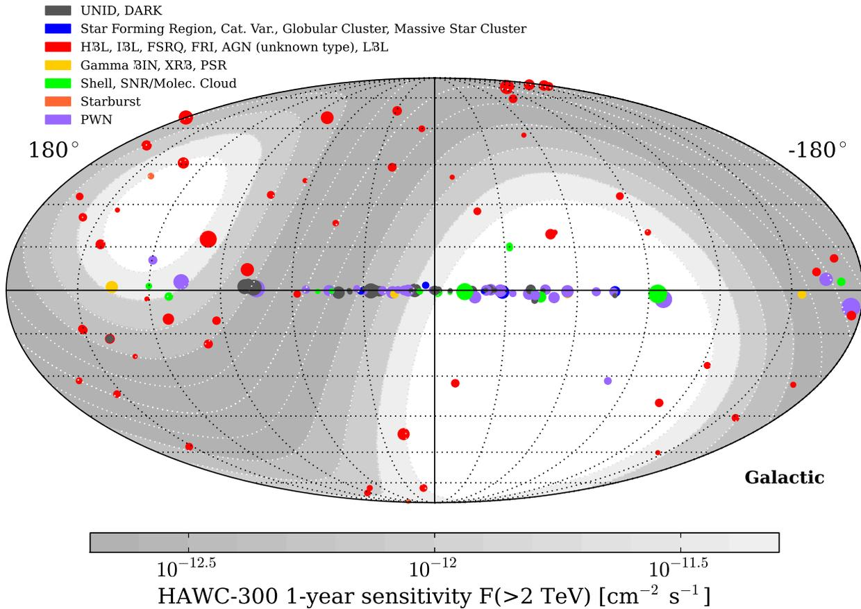
**Fig. 1:** The TeV sky visible to the HAWC observatory in Galactic coordinates. The detector sensitivity is declination dependent and darker grey bands indicate better sensitivity. Source classes of very-high gamma-ray emission as obtained with TeVCat[7] are overlaid.
