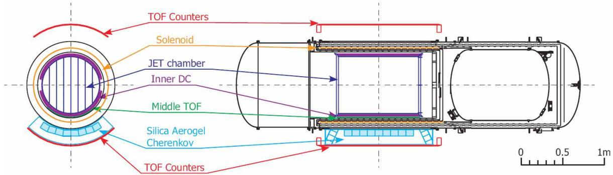
**Figure 2:** Cross sectional view of BESS-Polar II spectrometer
