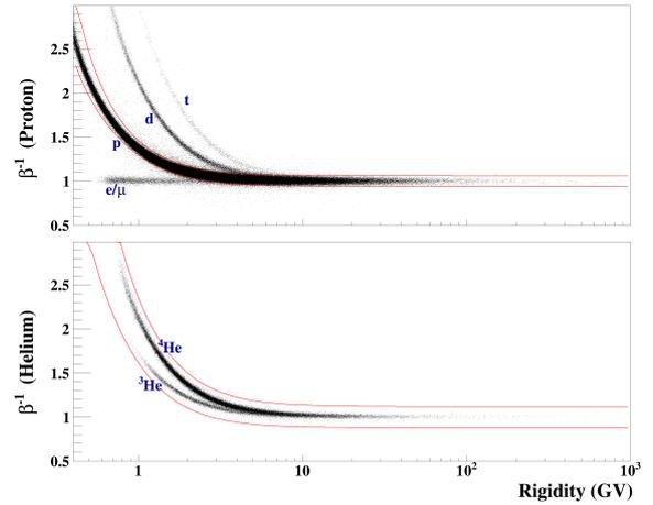
**Figure 5:** Scatter plot of  $\beta^{-1}$  vs. rigidity obtained from the balloon observation after proton and helium dE/dx selection.
