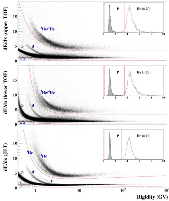
**Figure 4:** Proton band in dE/dx (top: upper TOF, middle: lower TOF, bottom: JET) vs. rigidity obtained from the balloon observation. The superimposed graph shows the selection criteria for protons and helium nuclei above 10 GV.
