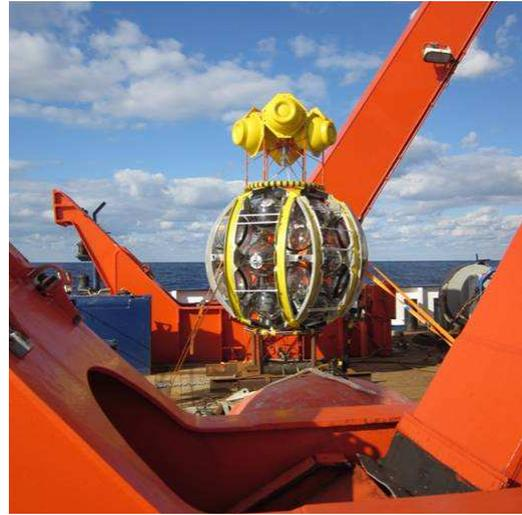
**Figure 2:** Photograph of the launcher vehicle on board the ship Meteor with a mockup of a string.
