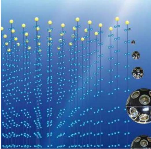
**Figure 1:** Artist impression of the KM3NeT detector. On the right, a zoom in of the optical module.
