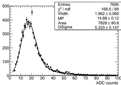
**Figure 2:** Typical distribution of MIP signal in an ECAL cell.
