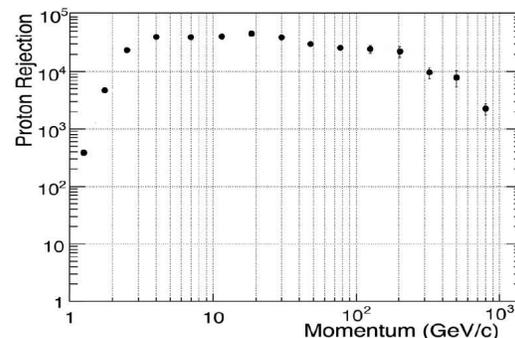
**Figure 7:** Proton rejection using ECAL BDT and an Energy/Rigidity cut (>0.75). Electron efficiency is 90%.
