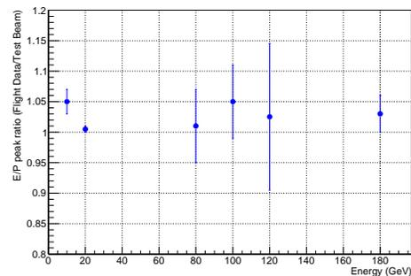
**Figure 4:** Ratio of Energy/Momentum ratio in flight and at 2010 Test Beam. Errors are dominated by beam statistics.
