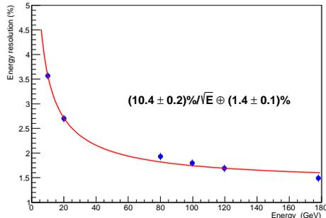
**Figure 5:** ECAL energy resolution measured at 2010 Summer test beam.
