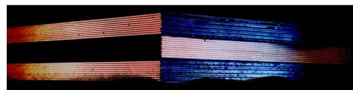
**Figure 1:** ECAL active part structure: lead and fiber layers are alternated; each 10 fiber layers (*superlayer*) the fiber orientation is rotated by 90 degrees.
