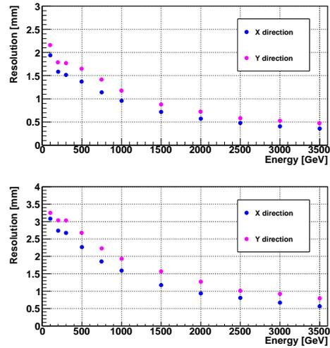
**Figure 3:** Position resolution for neutrons as a function of energy. Upper and lower panel correspond to the resolution of small tower and large tower, respectively.
