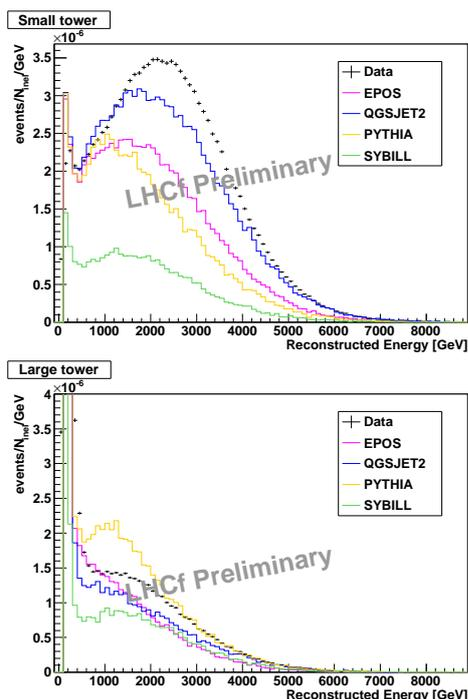
**Figure 8:** Measured energy spectra of neutron-like events together with the MC predictions. Upper and bottom panels are the results for the small tower and the large tower, respectively. The vertical bars represent the statistical uncertainties. Systematic uncertainty is not included.
