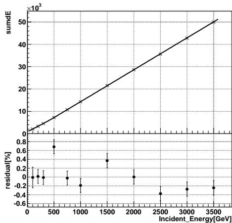
**Figure 4:** Energy response function. Upper panel shows the relation between the incident energy and means of sumdE. Black curve is a fitting result. Bottom panel shows residual from fitting.
