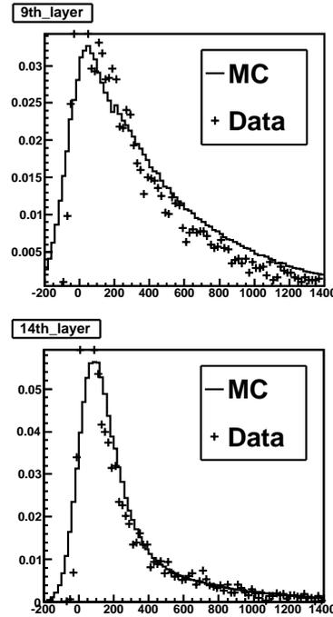
Figure 7: Deposited energy distribution of the 9th layer (upper) and the 14th (bottom) layer at the SPS beam test.
