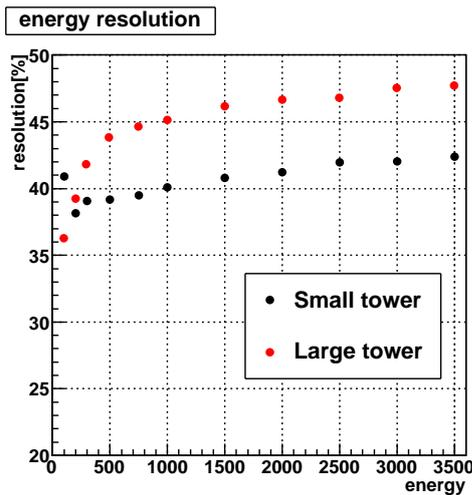
Figure 6: Energy resolutions of small tower (black) and large tower (red) for neutrons as functions of energy.
