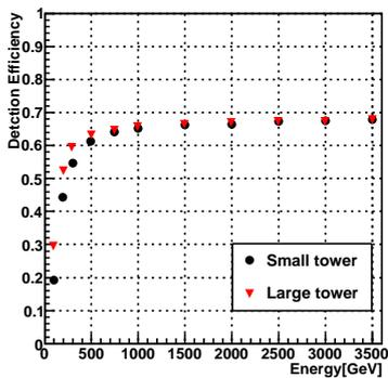
**Figure 2:** Detection efficiencies of neutrons as a function of energy. Black (Red) markers correspond to the efficiency of the small (large) tower.
