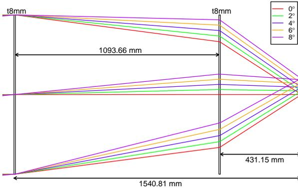
**Figure 3:** The optics design of the TA-EUSO.
