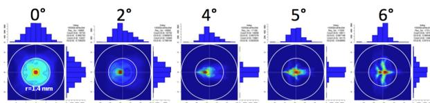
**Figure 6:** Spot diagrams of the EUSO-Balloon between FOV 0° and 6°. Inner circle radius is 1.4 mm. Outer circle radius is 2.8 mm.
