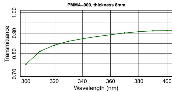
Figure 2: The 8mm thick PMMA transmittance in the near UV region.
