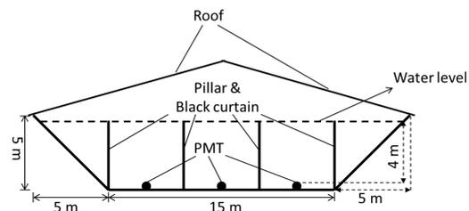
Fig. 1: The structure of the engineering array.
