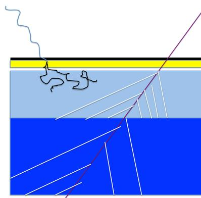
Figure 3: Multi-layered gamma observatory having a timing array and a EM layer and muon layer
