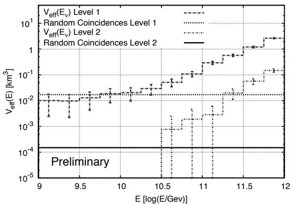
**Figure 4:** The effective volume of the AMADEUS detector as a function of the logarithmic neutrino energy for the two different levels, as described in the text. Also shown are the random coincidence rates for the levels 1 and 2.
