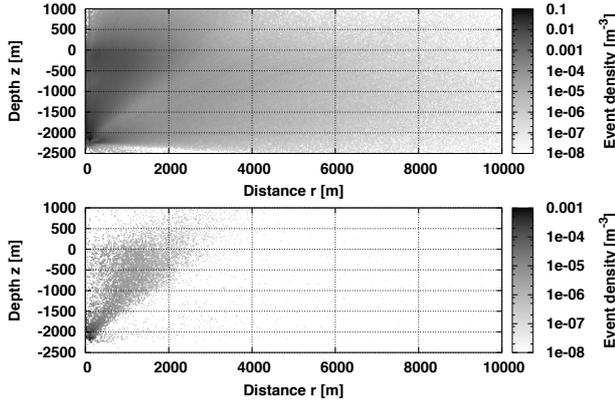
**Figure 3:** Spatial density of transient signals as a function of the depth  $z$  and the distance  $r$  from the centre of the AMADEUS detector. Top: the density of transient signals as selected by the AMADEUS online filter; bottom: events remaining after the offline cuts described in the text.
