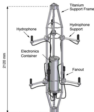
**Figure 2:** Drawing of a standard acoustic storey.
