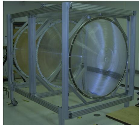
**Fig. 1:** The Bread-board model of the JEM-EUSO optics tested at MSFC, NASA, Huntsville. The diameter is 1.5 m.
