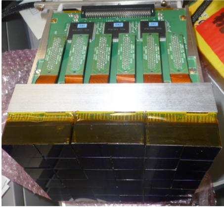
**Fig. 2:** The first prototype of the JEM-EUSO PDM, already integrated in RIKEN. It will be tested as the focal surface of the TA-EUSO experiment, to be deployed at the TA site in UTAH in summer 2013.
