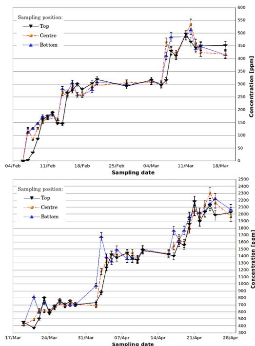
**Figure 2:** Gadolinium sulfate ( $\text{Gd}(\text{SO}_4)_3 + n \cdot \text{H}_2\text{O}$ ) concentration during Gd loading from three sample points: top, centre, and bottom of the 200-ton tank. The top figure shows single batch loadings while the bottom shows double batches.
