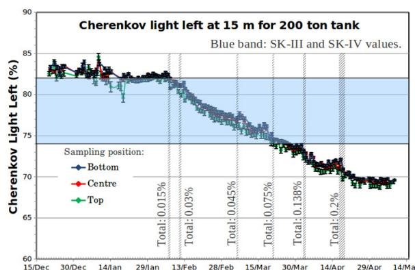
**Figure 3:** Water transparency in terms of percentage of Cherenkov light remaining after 15 meters of travel through the water in the 200-ton tank at three sampling positions: top, centre and bottom. Vertical hatched bands indicate Gd injections into the 200 ton tank and the horizontal blue band SK-III and SK-IV pure water values. Note the suppressed zero on the y-axis.
