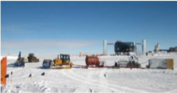
Figure 7: ARA hot water drill convoy in front of the Ice-Cube Laboratory, heading out to the field to drill 200m deep, dry instrumentation holes.
