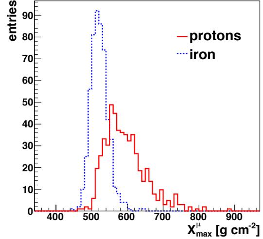
**Figure 1:**  $X_{\max}^\mu$  distributions for proton and iron showers simulated at 30 EeV with Epos-LHC [12] at zenith angles between  $55^\circ$  and  $65^\circ$ . The mean value and the RMS of the distributions show a clear dependence upon the mass of the primary cosmic ray. For the construction of these MPDs, only muons reaching ground at distances greater than 1700 m have been considered.
