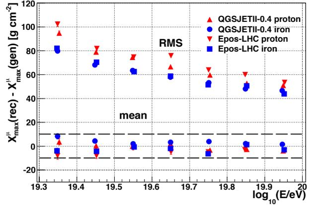
**Figure 3:** Evolution with energy of the RMS of the distribution  $[X_{max}^\mu (\text{reconstructed}) - X_{max}^\mu (\text{true})]$ . The simulations were made using the QGSJETII-0.4 [13] and EPOS-LHC hadronic models for proton and iron nuclei for  $55^\circ \leq \theta \leq 65^\circ$ .
