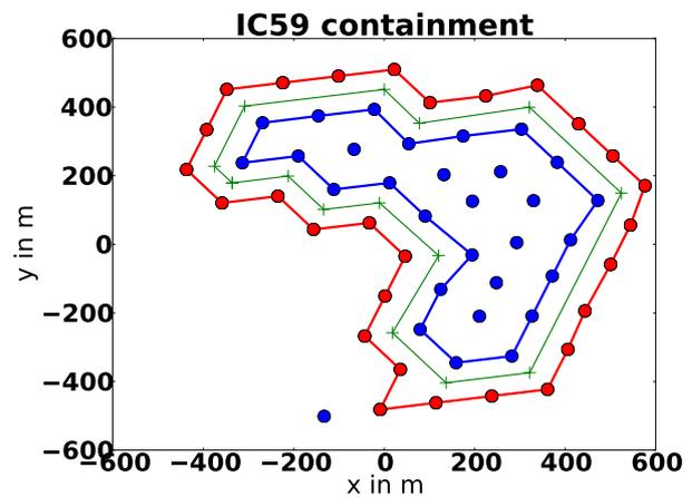
**Fig. 1:** Definition of containment in the x-y (horizontal) plane for the analyses presented here. Each dot represents an IceCube string, the outermost layer is marked by a red line, the second layer by a blue line, the green line is halfway between the two layers of strings. Analysis A requires the reconstructed event vertex to be within the area bounded by the green line, analysis B requires the reconstructed vertex to be within the red line.
