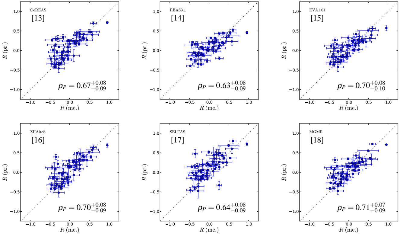
**Fig. 3:** Comparison of the  $R$ -parameters measured by AERA with six models for radio emission from extensive air showers. These calculations include the Askaryan charge-excess emission mechanism. The Pearson correlation coefficients and their 95% confidence levels quantify the level of agreement between simulation and data.
