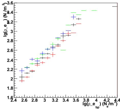
**Fig. 4:** Correlation between the electron densities measured by the four en-detectors of PRISMA-YBJ ( $\rho_{e_{pr}}$ ) and those measured by the four corresponding bigpads of ARGO-YBJ ( $\rho_{e_{bp}}$ ): D1(black), D2(red), D3(green) and D4(blue).
