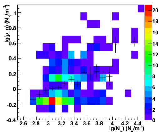
**Fig. 8:** Correlation between density of thermal neutrons detected by PRISMA-YBJ and the  $N_p$  value (energy estimator) as resulting from the fit of the lateral distribution in ARGO-YBJ with equation (1). Events with core within 10m from the PRISMA-YBJ center have been selected. Colors are number of events, and crosses are profile.
