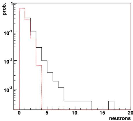
**Fig. 5:** Thermal neutron normalized distribution of the matched events (black solid line) and background normalized distribution (red dotted line).
