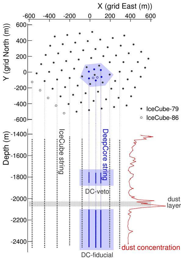
**Figure 1:** Top and side view of the IceCube detector (black) and its DeepCore subarray (blue). Strings constituting the IceCube 79-string configuration (solid) and the last deployed strings completing the IceCube detector (circles) are indicated. Also shown is the main dust layer within the detector and a dust concentration profile as measured with a dust logger [7].
