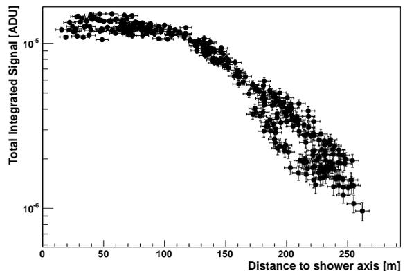
**Fig. 4:** Example signal strengths from a cosmic ray induced air shower as recorded with the LOFAR LBAs. The integrated signal per antenna is plotted against the distance to the shower axis as reconstructed from the particle data.
