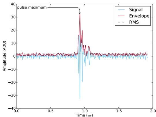
**Fig. 7:** A cosmic-ray induced pulse from the example event of figures 8 and 9 as reconstructed by the automated pipeline.
