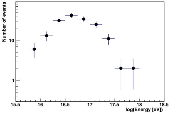
**Fig. 2:** Energies of all events triggered with the scintillator array, which have also been detected with a significant pulse in data in the low-band frequency range. The energy is the one reconstructed by the particle array, therefore quality cuts were applied.
