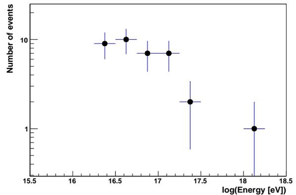
**Fig. 6:** Energies of all events (after cuts) triggered with the scintillator array, which have also been detected with a significant pulse in data in the high-band frequency range. The energy is the one reconstructed by the particle array, therefore quality cuts were applied.
