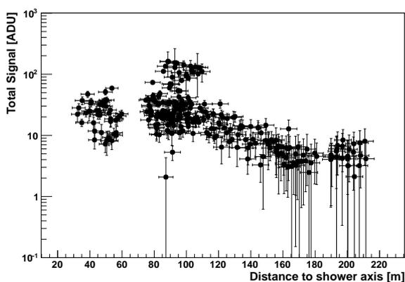
**Fig. 8:** Signal distribution of an example event as detected in the LOFAR high-band antennas. The total signal strength (peak amplitude) is shown as a function of distance to the shower axis. The uncertainty of the signal in the HBA is generally higher than the one in the LBAs due to instrumental effects.
