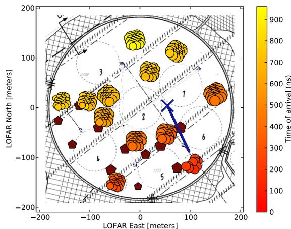
**Fig. 9:** Example event as detected in HBA. Shown is the most inner core of LOFAR. Every circle depicts an HBA tile and the dark red pentagrams correspond to the particle detector array. The size of the circles and pentagrams corresponds to signal strength and the colour of the circles indicates the time of arrival. Also shown is the reconstructed shower axis. Large empty circles are the location of the LBAs.
