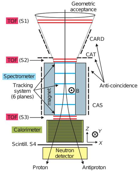
**Fig. 1:** A schematic overview of the PAMELA satellite experiment. The experiment stands  $\sim 1.3$  m high and, from top to bottom, consists of a time-of-flight (ToF) system (S1, S2, S3 scintillator planes), an anticoincidence shield system, a permanent magnet spectrometer (the magnetic field runs in the  $y$ -direction), a silicon-tungsten electromagnetic calorimeter, a shower tail scintillator (S4) and a neutron detector.
