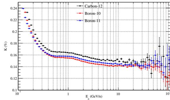
**Fig. 3:** Correction factor for particle lost due to inelastic scattering at the top of the payload.
