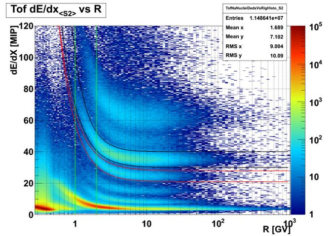
**Fig. 2:** Charge selection bands for boron (red) and carbon (black) on the mean energy release in S2 as a function of rigidity.
