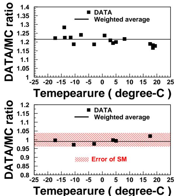
**Fig. 6:** Air fluorescence yield ratio  $R_{FK}$ (top) and  $R_{SM}$ (bottom) measured by the ELS.
