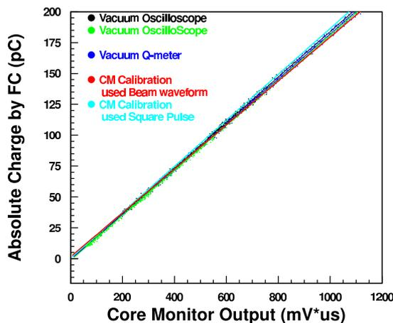
**Fig. 2:** Calibration of the CM. Plotted is a correlation between the integrated CM signal (X-axis) and the observed charge in FC or the supplied charge to the CM by calibration pulse (Y-axis).
