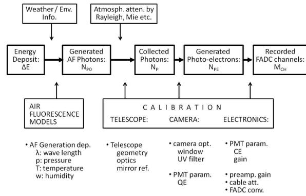
**Fig. 3:** Sequence of AF signal generation and detection.
