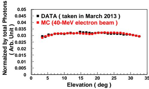
**Fig. 4:** Longitudinal distribution of AF photons from the ELS beam. One FD camera covers the elevation of  $3^\circ - 18^\circ$ , and another covers  $18^\circ - 33^\circ$ .
