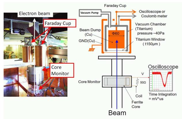
**Fig. 1:** Faraday Cup (FC) and Core Monitor (CM) for the ELS beam charge measurement.
