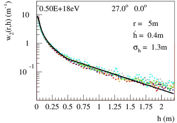
**Figure 3:** The distribution  $w_2(r, h)$  for  $r = 5$  m. The full black line represents the fit, the dotted lines are simulation results for different times. Figure taken from [14].
