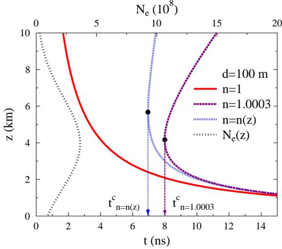
**Figure 1:** The emission height  $z = -\beta ct'$  as function of the observer time  $t$  for three different values of the index of refraction,  $n$ . The dashed black line gives the shower profile as function of  $z$  for a  $E = 5 \times 10^{17}$  eV proton-induced shower.
