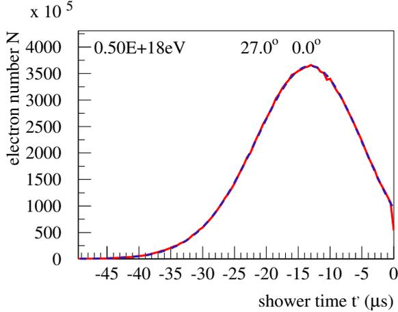
**Figure 2:** The number  $N$  of electrons and positrons, as a function of the shower time  $t'$ . The full red line represents the simulation result, the dashed blue line is the fit. Figure taken from [14].
