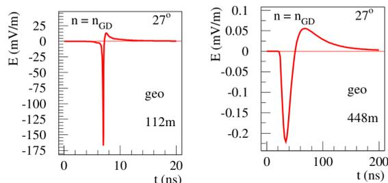
**Figure 6:** The geomagnetic contribution to the electric field for a  $5 \times 10^{17}$  eV, 27 degrees inclined shower observed at two different observer positions of  $d = 112$  meters (left) and  $d = 448$  meters (right) from the impact point of the shower. Figure taken from [14].
