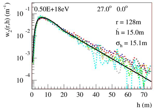
**Figure 4:** The distribution  $w_2(r, h)$  for  $r = 128$  m. The full black line represents the fit, the dotted lines are simulation results for different times. Figure taken from [14].
