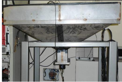
**Figure 4:** A scintillation counter to be deployed at Tunka-133.
