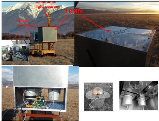
**Figure 5:** Photograph of one of the first 3 new optical stations.
