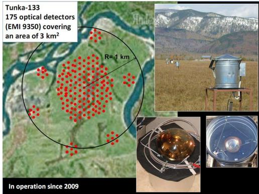
**Figure 1:** Layout of the Tunka-133 array.
