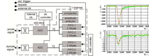
**Figure 2:** Internal structure of FADC board (shown only one channel, the second one is identical) (left). Example of signals from anode and dynode (right).
