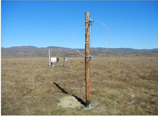
**Figure 3:** The Tunka-Rex antenna station in front of a cluster center and its central PMT
