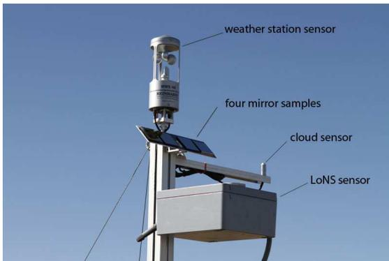
**Fig. 1:** The sensors of an ATMOSCOPE station
