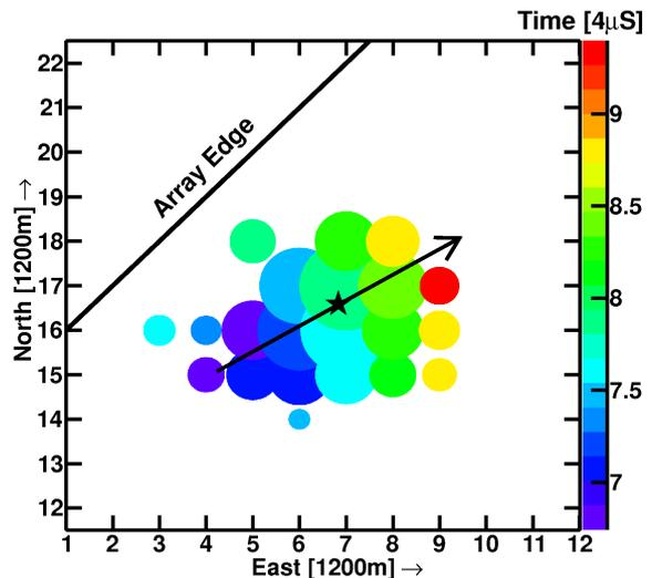
**Fig. 1:** A typical high energy event seen by the TA SD. Each circle represents a counter, positioned at the center of the circle, the area of the circle is logarithmically proportional to the counter pulse height, and the counter time is denoted by the color. The arrow represents the projection of the shower axis onto the ground, which we label by  $\hat{u}$ , and it is bisected by the perpendicular line at the location of the shower core.
