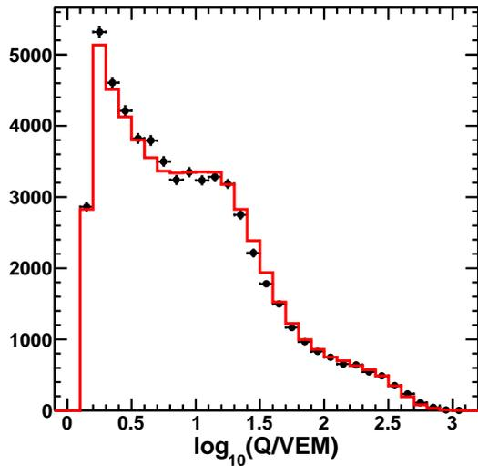
**Fig. 5:** Data and MC comparison of counter pulse height. The points with error bars represent the data histogram and the solid line represents the MC.
