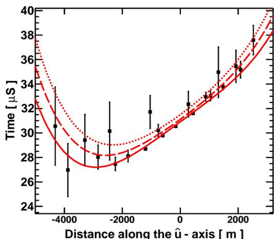
**Fig. 2:** TA SD time fit. Counter time is plotted versus the distance from the shower core along the  $\hat{u}$  direction, which is the projection of the shower axis on the ground. Points with error bars are counter times, solid curve is the time expected by the fit for the counters lying on the  $\hat{u}$  axis, dashed and dotted lines are the fit expectation times for the counters that are correspondingly 1.5 and 2.0 km off the  $\hat{u}$  axis.
