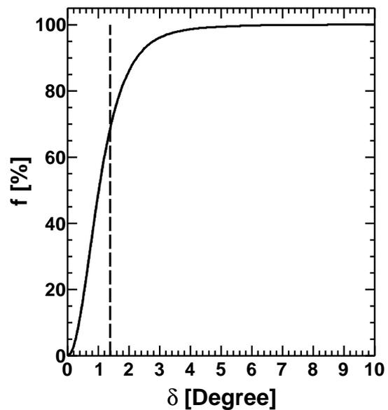
**Fig. 8:** Angular resolution of the TA SD evaluated by Monte-Carlo. Fraction of events ( $f$ ) reconstructing within a certain opening angle ( $\delta$ ) of the true event direction is plotted versus the opening angle. 68% of events reconstruct within  $1.4^\circ$  of the true event direction.
