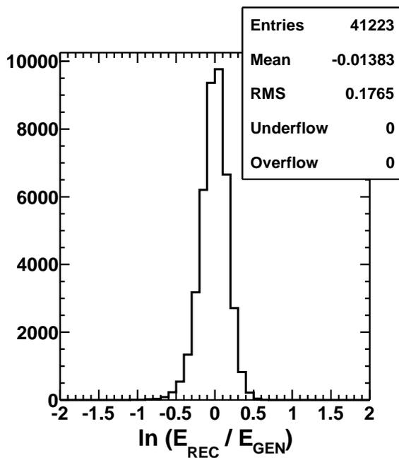
**Fig. 9:** Energy resolution of the TA SD evaluated by the Monte-Carlo. The histogram shows the distribution of the natural logarithm of the reconstructed ( $E_{\text{REC}}$ ) energy divided by the true energy ( $E_{\text{GEN}}$ ).
