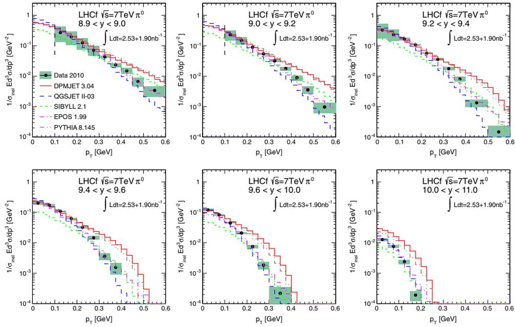
**Fig. 2:** Transverse momentum spectra of forward  $\pi^0$  in each rapidity bin. The black dots and the shaded area show LHCf data and the uncertainties. The color lines indicate the predictions by several hadron interaction models [13, 14, 15, 16, 17].
