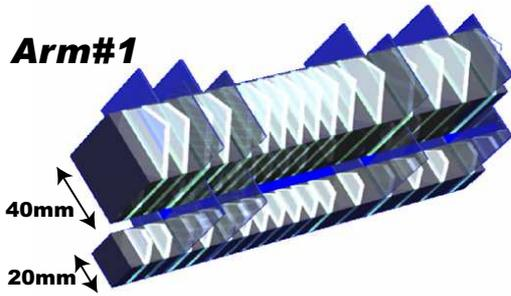
Fig. 1: Schematic view of the LHCf-Arm 1 detector
