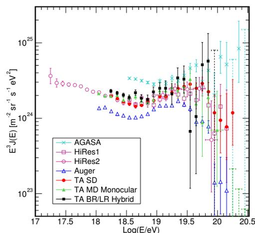
**Fig. 5:** The energy spectra multiplied by  $E^3$ . The spectrum determined from the hybrid data is shown by the black boxes. The spectra of AGASA [18], HiRes-1/HiRes-2 [7], Auger [19], TA SD [20] and TA MD [21] are also shown for comparison.
