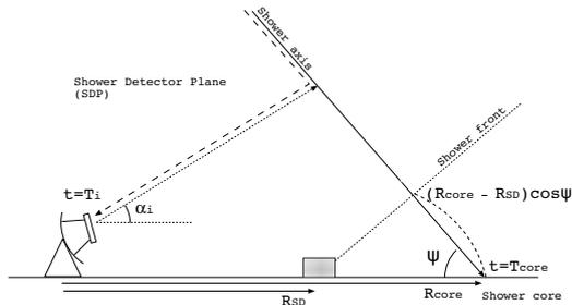
**Fig. 1:** Diagram indicating the Shower Detector Plane (SDP) for use in the time fit.
