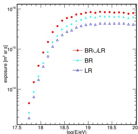
**Fig. 4:** The calculated hybrid exposure as a function of the energy of the cosmic ray primary.
