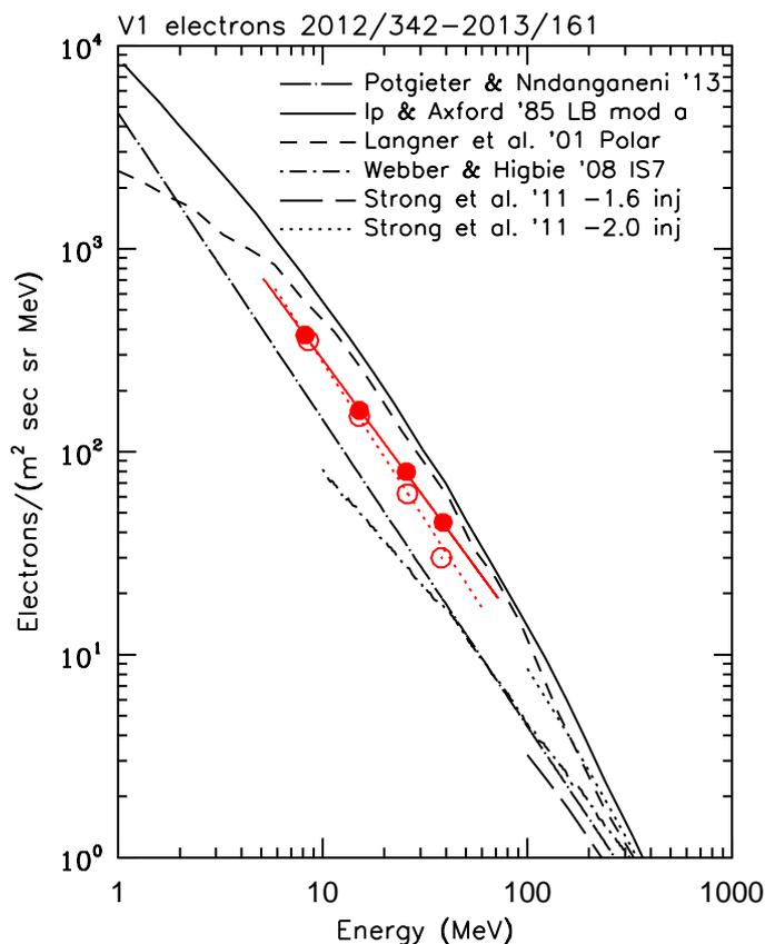
**Figure 4:** Differential energy spectrum of electrons from V1 for the period 2012/342-2013/161. The open symbols represent analysis done using response functions derived from a pre-flight calibration at an electron accelerator. The solid symbols represent the energy spectrum derived from a simulation using the Geant4 software ([www.geant4.cern.ch](http://www.geant4.cern.ch)). The differences between the results of the two methods gives an indication of the systematic uncertainty.
