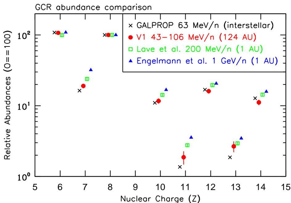
**Figure 3:** GCR abundances relative to O from the V1 observations in the energy range 43-106 MeV/nuc for the period 2012/342-2013/161 compared with those at higher energies [3, 9] at 1 AU where there is significant solar modulation. Also shown are the interstellar estimates from a GALPROP conventional diffusive reacceleration model that was tuned to ACE data at 1 AU by [9].
