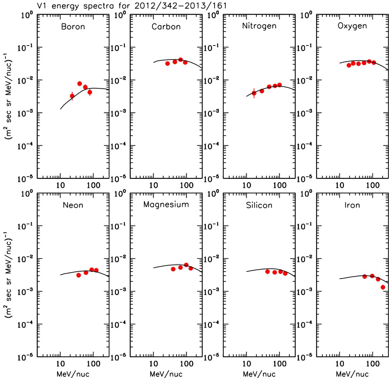
**Figure 2:** Preliminary differential energy spectra from V1 for the period 2012/342–2013/161. The line is a GALPROP conventional diffusive acceleration model that was tuned by [9] to fit ACE data at higher energies at 1 AU. The GALPROP results file is [http://galprop.stanford.edu/wrxiv/results\\_54\\_0572000f\\_4fdgrmny7ffy65y.tar.gz](http://galprop.stanford.edu/wrxiv/results_54_0572000f_4fdgrmny7ffy65y.tar.gz).
