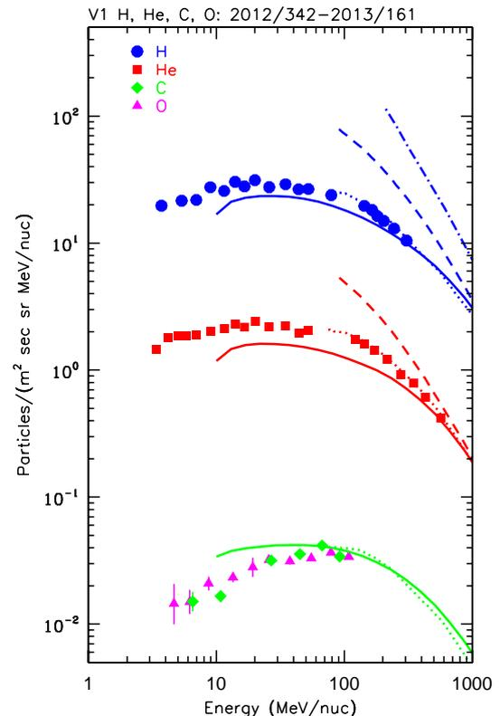
**Figure 1:** Differential energy spectra from V1. Estimates of the interstellar GCR spectra are shown and discussed in the text: GALPROP model (solid line); leaky box model [20] (dotted); DC model [10] (dashed); and pump acceleration model [4] (dot-dash).
