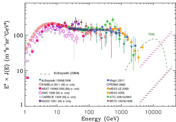
**Fig. 1:** All-electron energy spectrum measurements to date. The UHE flux from Vela predicted by one set of model parameters, described in [2], is shown as a dashed line. The top hatched line shows the anticipated CREST sensitivity for the recently completed 10 day flight, while the bottom hatched line shows that for a 50 day flight.
