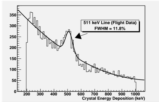
**Fig. 5:** Fit to the 511 keV annihilation line observed in flight.
