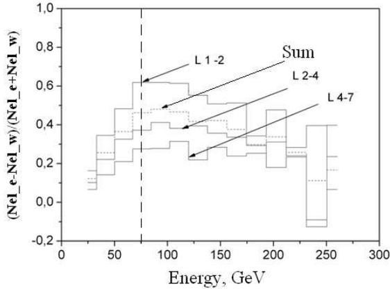
**Fig. 3:** The estimated  $(Nel_e - Nel_w)/(Nel_e + Nel_w)$  for electrons as a function of the electron energy. The dotted line shows where an influence of protons can be neglected.
