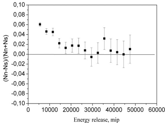
**Fig. 5:**  $(Nn-Ns)/(Nn+Ns)$  as a function of the total energy release inside the calorimeter.
