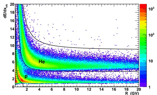
**Figure 1:** Energy released in the PAMELA tracker system by hydrogen and helium particles as a function of the particle rigidity.
