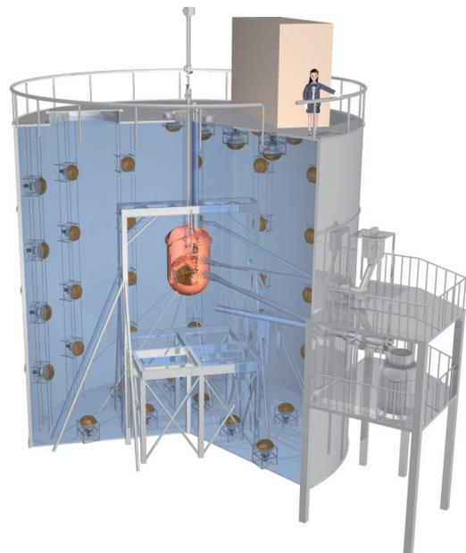
**Fig. 1:** Water tank for radiation shield against neutrons and gamma rays from the rock. The size is  $\phi$  10 m  $\times$  H 10 m and the vacuum insulated OFHC Copper vessel which holds liquid xenon was mounted in the center.
