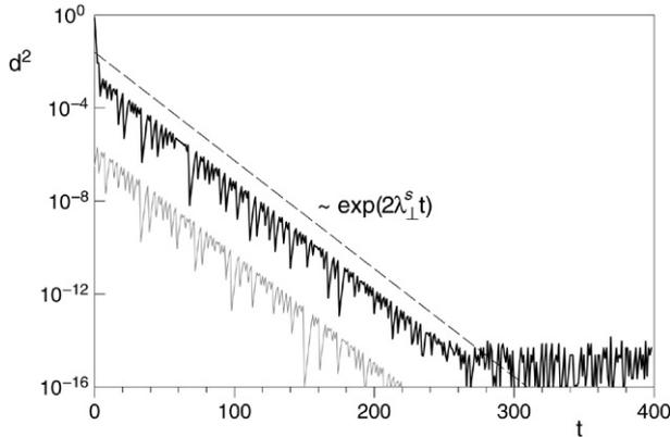
Fig. 4. Relaxation to the synchronization manifold. Time series of  $d^2$  for the same CML of Fig. 1 with  $\alpha = 0.8$  (subcritical). The dashed line corresponds to the exponential law indicated in the figure, for comparison. The gray line corresponds to a realization of Eq. (10).
