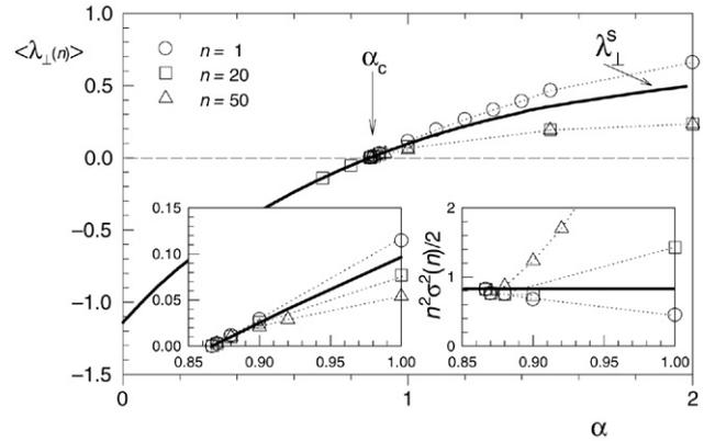
Fig. 2. Average  $n$ -step exponents as a function of  $\alpha$  for the same CML of Fig. 1. Left side inset: zoom around critical values. Right side inset: scaled standard deviation. In all cases full lines correspond to the asymptotic value in synchronous states.
