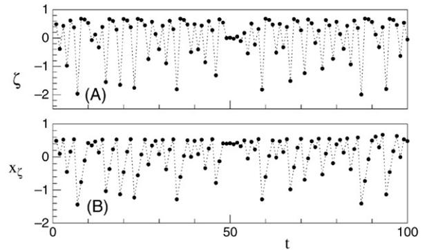
Fig. 3. Time evolution of  $\zeta = \lambda_{\perp}(1) - \lambda_{\perp}$  (A) and  $x_{\zeta} = \sum_{t=1}^t \zeta(t)$  (B) for the same CML of Fig. 1 with  $\alpha = 0.9$  (supercritical).
