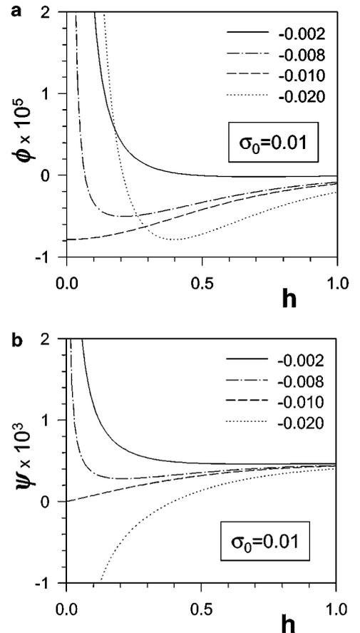
FIG. 2. Potentials of the operative forces. (a) Disjoining pressure  $\phi$  (Eq. [3]) and (b) electric surface potential  $\psi$  (Eq. [4]), as a function of the film thickness  $h$  for different values of the electric charge density  $\sigma_s$  of the substrate (indicated on the figure) and charge density of the vesicle  $\sigma_0 = 0.01$  ( $\kappa = 10/3$ ).
