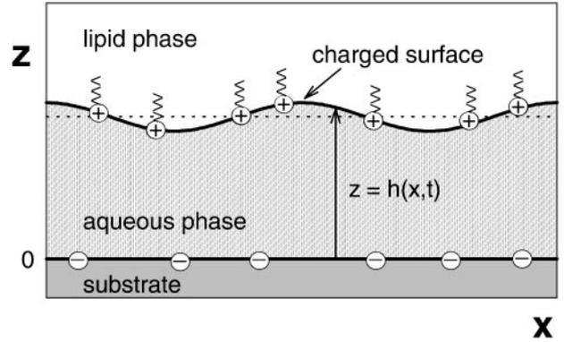
FIG. 1. The system: a thin aqueous film is bounded by a fixed substrate and by a free surface which delimits a lipid phase. The substrate and the free surface have electric charge densities of opposite sign ( $\sigma_s$  and  $\sigma$ , respectively). The free surface is described by  $z = h(x, t)$ .
