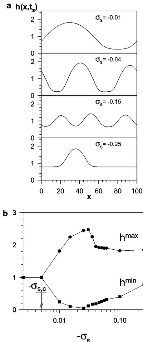
**FIG. 6.** Profile wavelength and amplitude dependence on the support charge  $\sigma_s$ . (a) Film thickness profiles  $h(x, t_s)$  as a function of  $x$  at a time  $t_s$  belonging to the first plateau of  $h^{\max}(t)$  as in Fig. 5b, for various values of  $\sigma_s$  indicated on the figure. All other parameters as in Fig. 4. (b) Maximal and minimal values of the film thickness at a time  $t_s$  as a function of  $\sigma_s$ .
