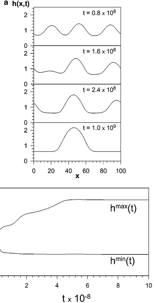
**FIG. 5.** Multiplicity of the steady state solutions and wavelength selection. (a) Shapes of the film surface  $h(x, t)$ , obtained from numerical integration, as a function of  $x$  at various times  $t$  indicated on the figure. All parameters are as in Fig. 4 except for  $\sigma_s = -0.15$ . (b) The temporal behavior of the minimal and maximal values of  $h(x, t)$ .
