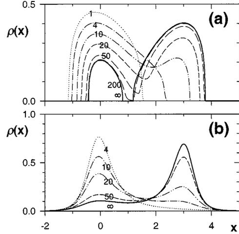
FIG. 5. Time evolution of the density of particles obtained by numerical integration of Eq. (2) with  $\rho(x,0) = \delta(x)$  for  $(\nu, D) = (4.0, 2.5)$  (a) and  $(0.5, 0.1)$  (b). The profiles correspond to times  $t$  indicated in the figure.
