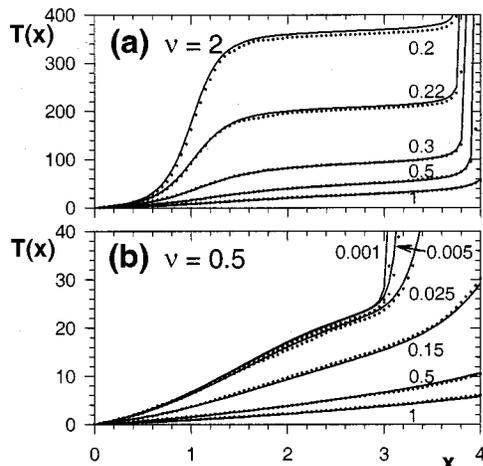
FIG. 3.  $T(x) \equiv T(x_L \rightarrow x)$  vs  $x$  for different values of  $D$  indicated in the figure and  $\nu = 2$  (a) and  $0.5$  (b). Circles correspond to numerical experiments (mean value over 1000 realizations) and full lines to theoretical prediction given by Eq. (6).
