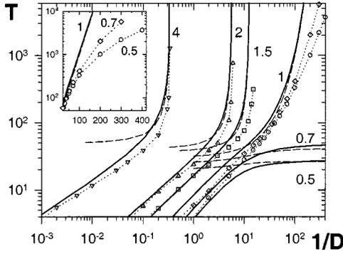
FIG. 4. Escape time  $T \equiv T(x_R)$  as a function of  $1/D$ , for different values of  $\nu > 0$  indicated in the figure. Full lines are generated from Eq. (6). Dashed lines correspond to the low- $D$  approximation given by Eq. (7). Symbols correspond to the initial condition where all the particles (at least 1000) are injected at the same time at  $x_L$ . Dotted lines are guides for symbols. Inset: Detail (semilog) of the low- $D$  region for  $\nu \leq 1$ .
