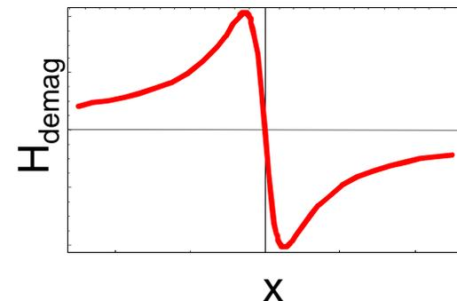
demag. field profile from the center of an isolated transition
