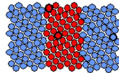
The smaller bits have a higher probability of flipping and the data is unstable
