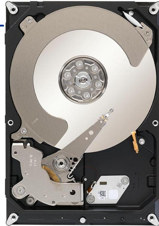
*“The actuator arm and suspension of the rotary actuator are collinear making the movement of the slider follow an arc and not a straight line.”*
