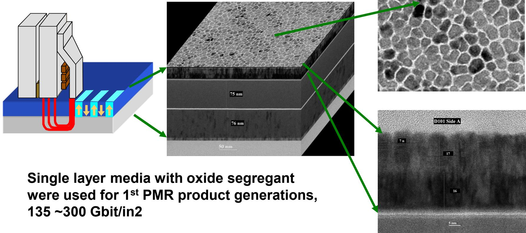
Single layer media with oxide segregant were used for 1<sup>st</sup> PMR product generations, 135 ~300 Gbit/in<sup>2</sup>
