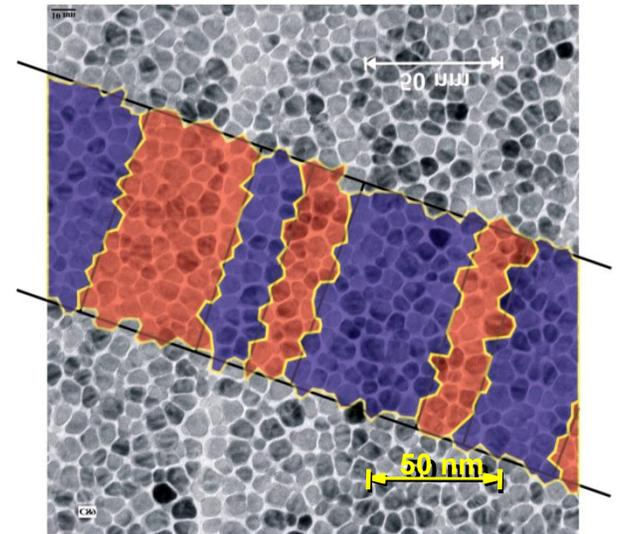
$$\text{SNR}_{\text{media}} \propto \sqrt{N} \quad N: \# \text{ of grains/bit}$$
