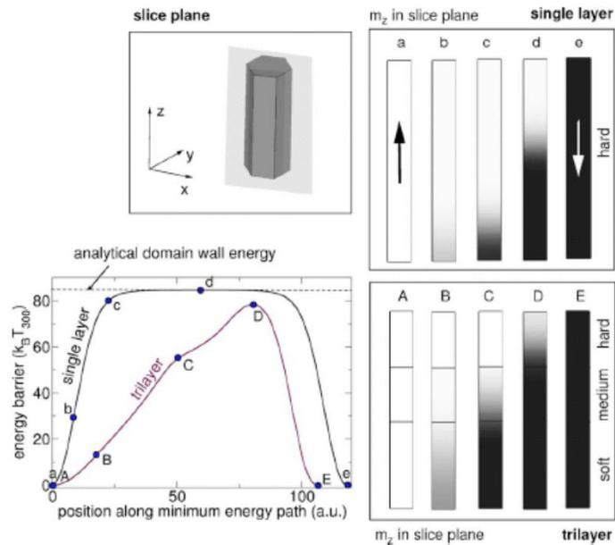
FIG. 3. Energy barrier and thermally activated switching process for a single phase media and the trilayer of Fig. 1. The hardest layer of the trilayer is 7 nm. The grain diameter is 5 nm. The  $z$  component of the magnetization during thermally activated switching is color coded.
